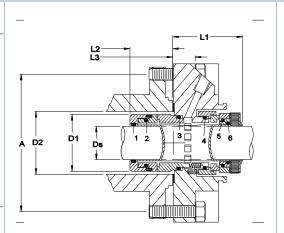
Optional exotic metal gland insert for corrosive environments. (Hastelloy "C", "B", Titanium, etc.)
