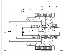
Optional exotic metal gland insert for corrosive environments. (Hastelloy "C", "B", Titanium, etc.)
