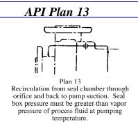
A line is connected from the pump suction to the seal gland. This is used to reduce pressure in the seal chamber enabling the seal to run cooler and to recirculate liquid and solids away from the seal faces.
