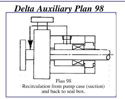
A line is connected from the pump suction to the stuffing box / seal chamber. This is used to reduce pressure in the seal chamber enabling the seal to run cooler and to recirculate liquid and solids away from the seal faces.
