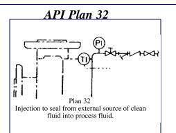
The seal is flushed from a clean, cool external source at a rate and temperature to maintain a proper environment for the seal. The flush must be sufficient to prevent the pumped fluid from entering the seal chamber. A close clearance bushing installed in the bottom of the seal chamber will reduce the flush required by increasing the velocity at the throat at a given flow.
