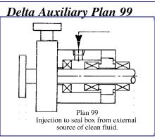
The seal is flushed from a clean, cool external source at a rate and temperature to maintain a proper environment for the seal into the stuffing box / seal chamber. The flush must be sufficient to prevent the pumped fluid from entering the seal chamber. A close clearance bushing installed in the bottom of the seal chamber will reduce the flush required by increasing the velocity at the throat at a given flow.
